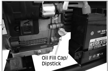
4. Replace the oil fill cap/dipstick and finger tighten securely.
